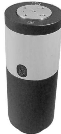
Converts the charge output from the AP Tech piezoelectric transducers to a low-impedance voltage output. The converter-input connects directly via a 10-32 microdot-connector to the cable of the vibration transducers; the output signal is available from a standard BNC-connector. AP5000 is powered over the signal-line from a constant current source such as found in most modern signal-analyzers.
