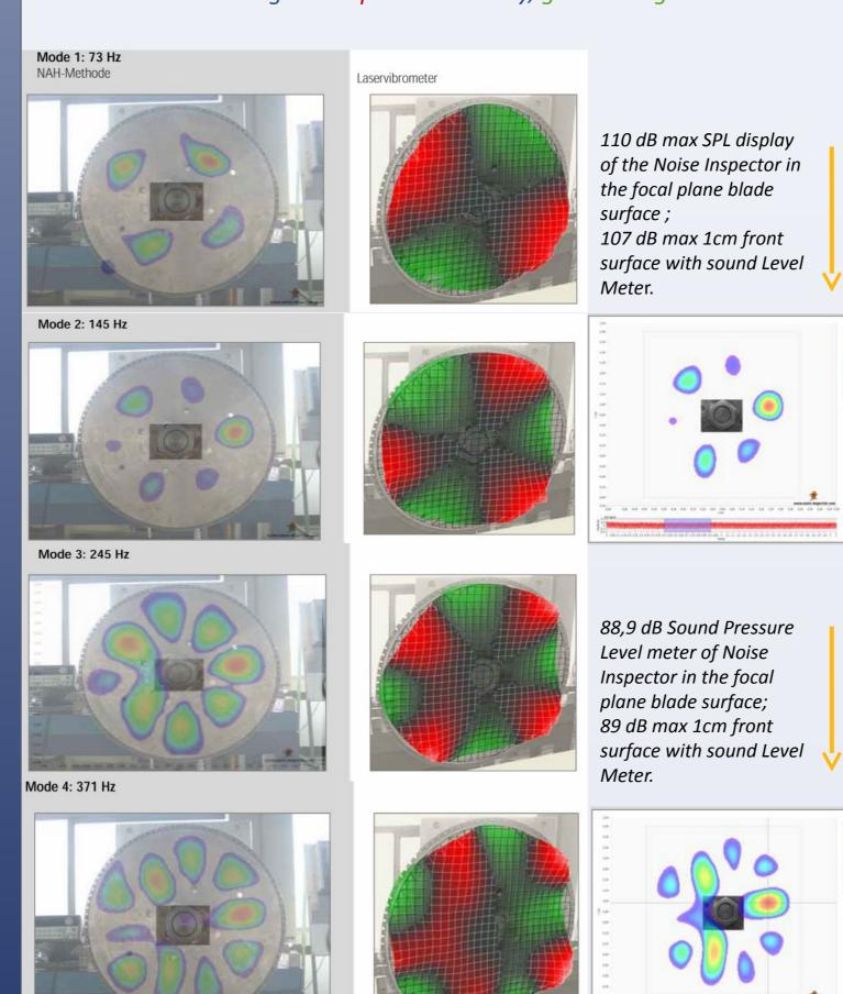
Number and location of sound sources match the locations at which the vibration velocity-speed of the blade surface has its maxima. For Mode 2 and Mode 4, it also reported the map of sound pressure level measured with a sound level meter, which can be compared with noise level map obbtained with the NAH Noise inspector. The NAH process works here up to frequencies of 73 Hz The use of beam forming method is usually demonstrating this limited to frequencies above 800Hz
