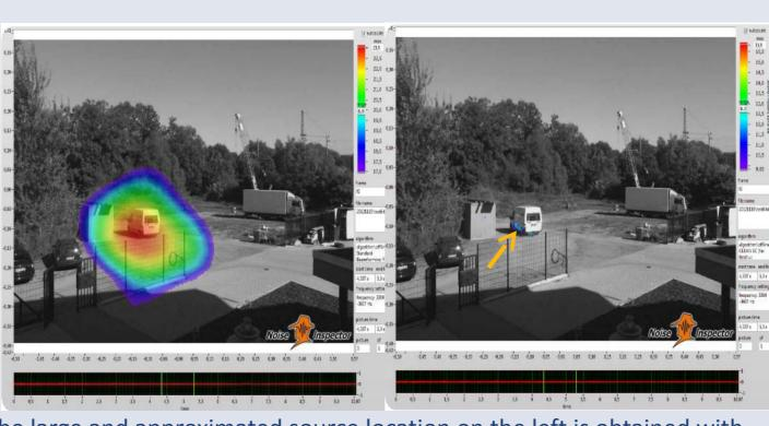
The large and approximated source location on the left is obtained with standard beamforming, while on the rigth is can be seen the powerfull performance of the Clean-SC to perfectly localize the source (arrow indication).
