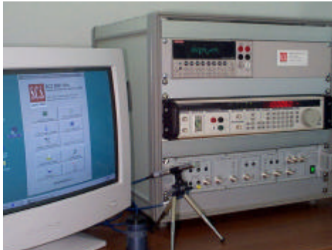
SCS 9001 test bench typical setup
