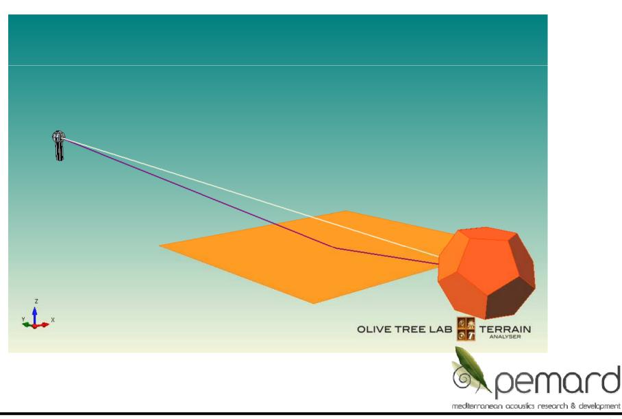
CORRECTED FOR REFLECTING SURFACE SIZE USING FRESNEL ZONES CORRECTION
